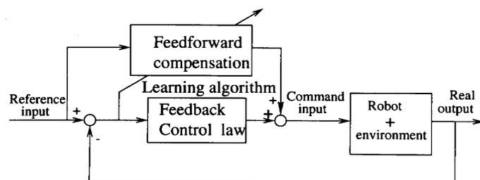
Fig. 13. Schematic drawing of robot learning position/force control.
