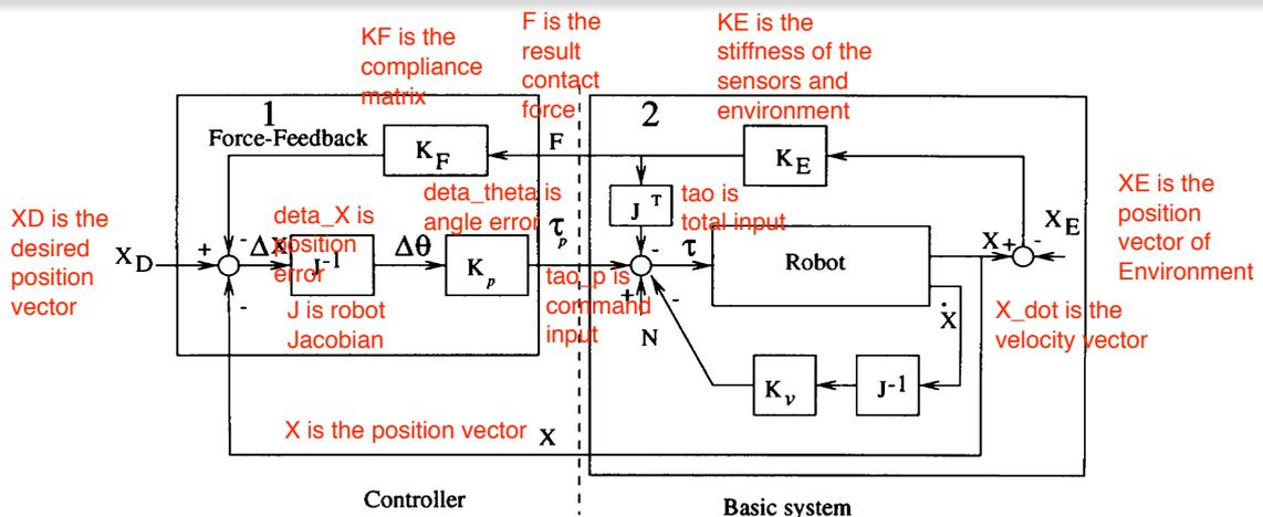
Fig. 1. Active stiffness control, version one.
