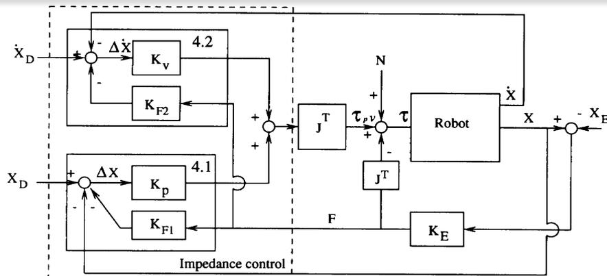
Fig. 3. Basic impedance control.
