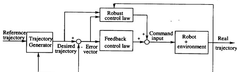
Fig. 12. Robot robust force control.
