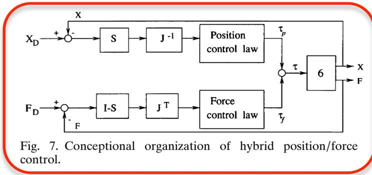
Fig. 7. Conceptual organization of hybrid position/force control.
