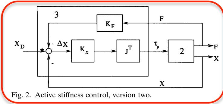
Fig. 2. Active stiffness control, version two.
