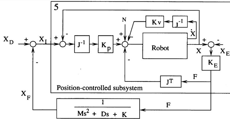
Fig. 4. Position-based impedance control.
